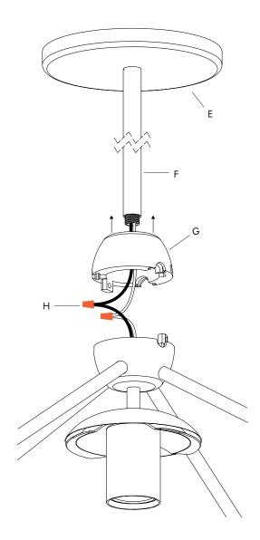
9. Secure the two half hubs together using a hex key and the provided #8-32 socket screws on either side.
