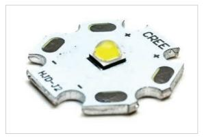
Used in the Rhea, ALO and LED Thin, the Cree LED produces beautiful, even colour. The Rhea pendant produces 360 Lumens, the ALO produces 100 Lumens while the LED Thin delivers 750 Lumens.
