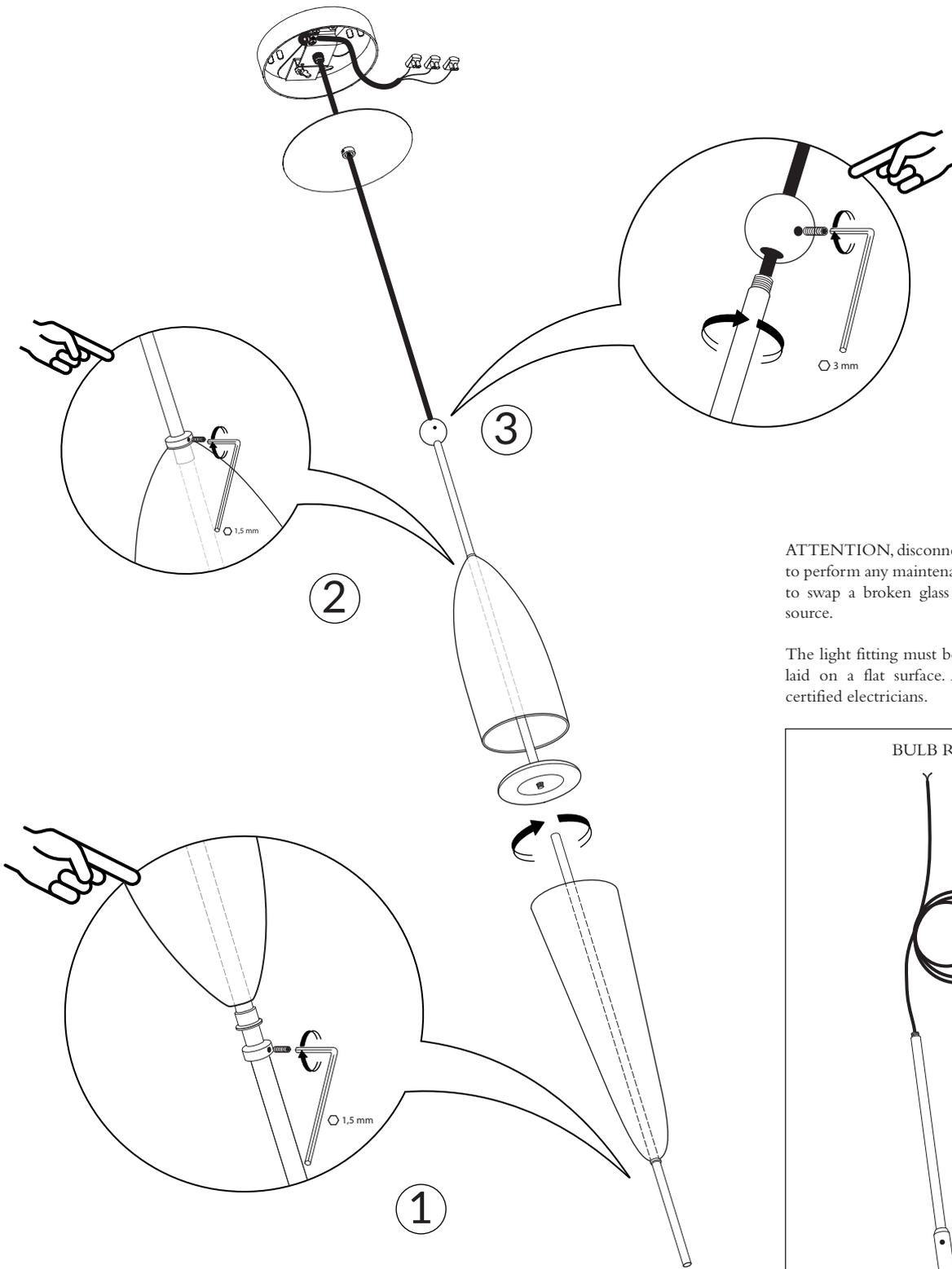
ATTENTION, disconnect the light fitting from the ceiling to perform any maintenance operation. In PARTICULAR, to swap a broken glass shape and/or swap a faulty light source.
